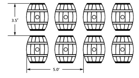
If space is available to have aisles so the wine can be worked in place, the aisles should ideally be wide enough to accommodate a ladder. Climbing between the stacks is not recommended, but it is done, particularly with stacks only 3 or 4 barrels high. An additional 12" space over that for the close-pack senario is adequate for climbing the stacks. Barrel density for this case is shown in the table in the rows marked "12+inch aisles".
