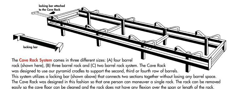
The stainless steel Cave Rack comes with foot pegs or variable height rubber feet. The barrels rest on the standard Western Square cradles and each barrel is about 5" apart (depending on the cooper) allowing the cellar crews the ability to work the barrels in place. This is an alternative solution to the Western Square traditional barrel racks.
