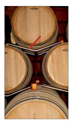
Western Square has two handy devices for stacking a single barrel above tiers of two barrels. One is the pyramid stacking cradle (pictured left) and the other is the center cradle (pictured right).
